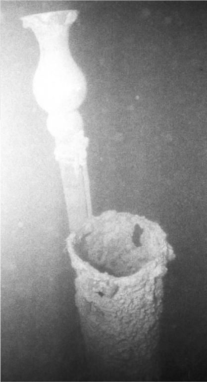
The funnel, with the top section missing, and the safety valve tube, the latter partly damaged by oxidation, on the E. Nordevall. The top section of the funnel seems to have fallen down already before the localization of the vessel and is today lying on the deck beside the funnel itself (Kent Hult).
