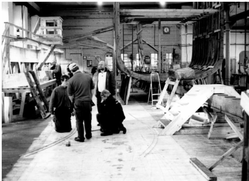
The master shipwright and his colleagues discussing the lines of the ship on the frame floor. The hull of the replica under construction is in the background (Photo: Carl Olof Cederlund).
