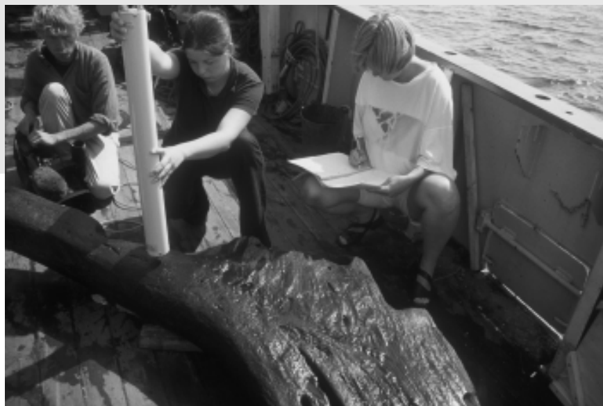
Examining the deck knee with a device measuring the bore resistance. Photographer: Roland Obst, Erfurt.
