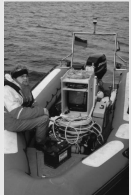
Preparing the georadar. The scuba radar antenna with the video camera as well as a screen for observation can be recognized. Photographer: Matthias Orgeldinger, Nürnberg.
