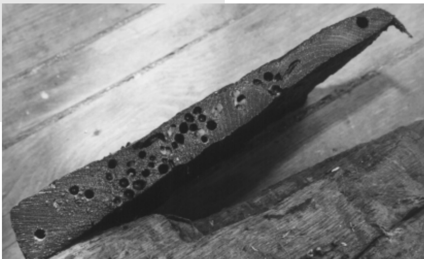
The destructive effect of Teredo navalis is shown on this sawn-open plank. Photographer: Matthias Orgeldinger, Nürnberg.
